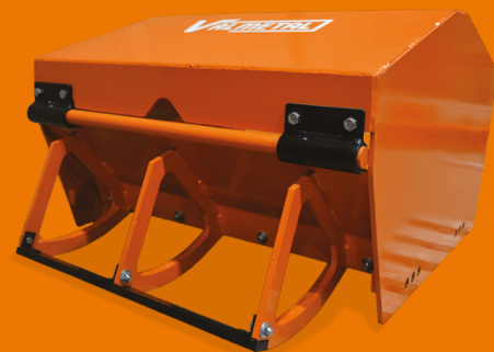
The 24" or 36" (61 or 91 cm) wide scraper box is equipped with large 8" (20 cm) wear plates made of 1/2" (13 mm) thick AR steel. Its bolted runners and tilting door are easily replaced.
