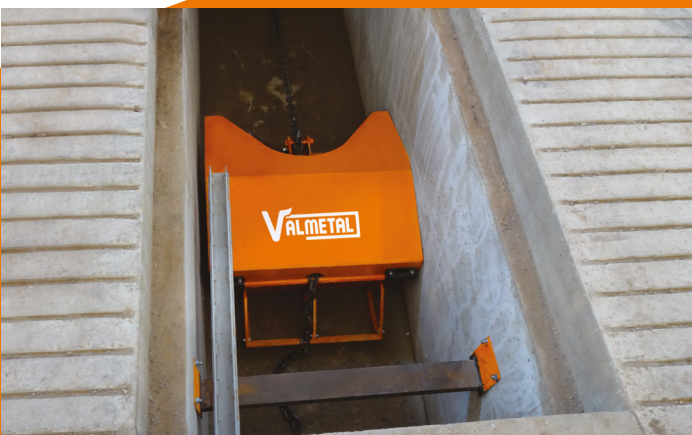
The 24" or 36" (61 or 91 cm) wide scraper box is equipped with large 8" (20 cm) wear plates made of 1/2" (13 mm) thick AR steel. Its bolted runners and tilting door are easily replaced.
