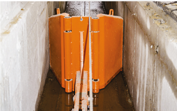
The 22" (56 cm) high V-Scraper can accommodate gutters of 24", 36" or 48" (61, 91 or 122 cm), variable width.
