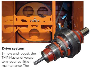
final chain drive is powered by a high-efficiency planetary drive with 4" (10 cm) diameter output shaft. Its large roller chains are self-lubricating in the oil bath and the bank of grease fittings is easy to access.
