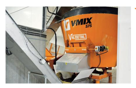
The **400** and **575** are the most popular models of the V-MIX series. The unique shape or their tub features a flat side that greatly speeds bale shredding which offers an appreciable time and energy saving day after day.
