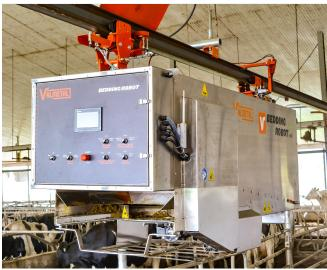
A programmable controller automatically manages the loading and distribution of bedding into stalls or pens.
