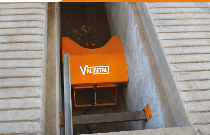
The Scraper box of 24" or 36" (61 or 91 cm) wide is equipped with large 8" (20 cm) wear plates made of 1/2" (13 mm) thick AR steel. Its bolted runners and tilting door are easily replaced.
