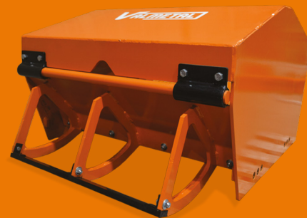
The Scraper box of 24" or 36" (61 or 91 cm) wide is equipped with large 8" (20 cm) wear plates made of 1/2" (13 mm) thick AR steel. Its bolted runners and tilting door are easily replaced.
