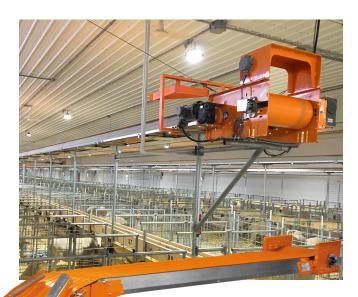
The large diameter drive rollers are covered with a non-slip rubber for positive belt traction.
