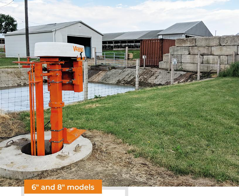
The 6" and 8" (15 and 20 cm) Vertical transfer pumps are designed for wastewater, hog manure or other non-bedded liquid manures. The rubber lower bearing withstands milkhouse chemicals and silo leachate, making these pumps the ideal choice for these tough jobs. For use in thin liquids / maximum slump test of 1/4" (6 mm).
