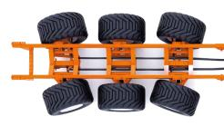
Non-steerable tankers tear up the headlands and roads while Maxx-Trac tankers roll smoothly through corners.
